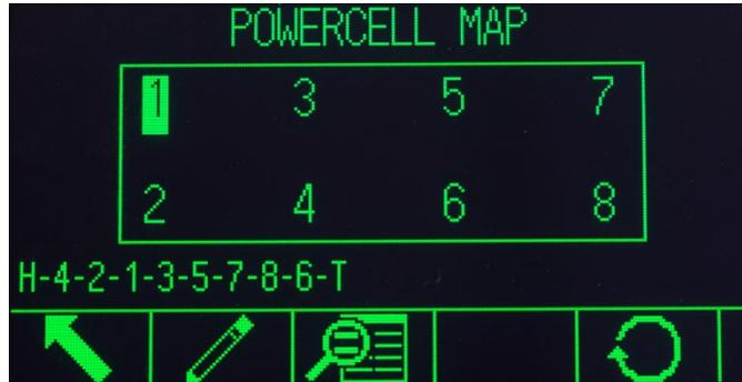
**Figure 3-35: Completed POWERCELL Load Cell Map**
