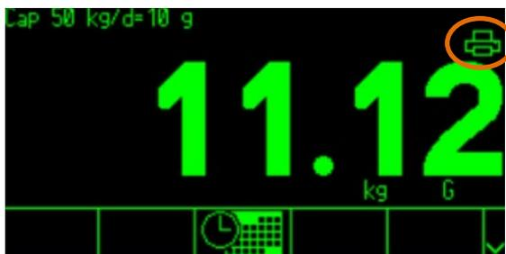
**Figure C-5: Printer Connection Status in System Line**
