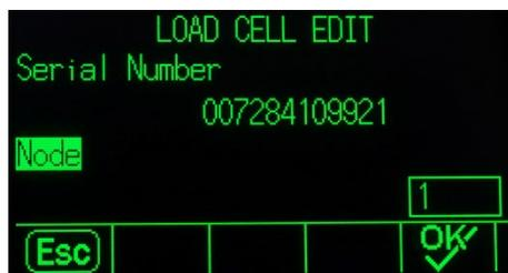
**Figure 3-12: Manual Address Load Cell Edit Screen**
