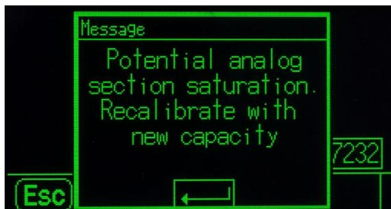
Figure 3-8: Analog Saturation Warning
