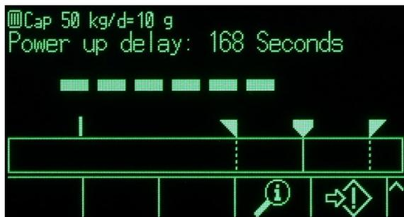
**Figure 3-6: Power Up Delay Shown in System Line**
