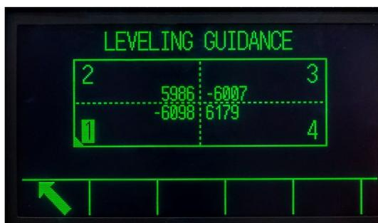
**Figure 5-6: Leveling Guidance Graphic Display**
