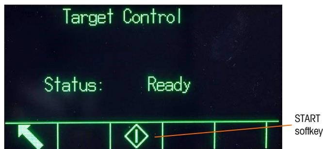
**Figure 2-19: Example of Ready State in Target Control**
