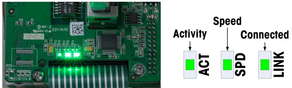
**Figure 5-10: Ethernet TCP/IP LEDs**
