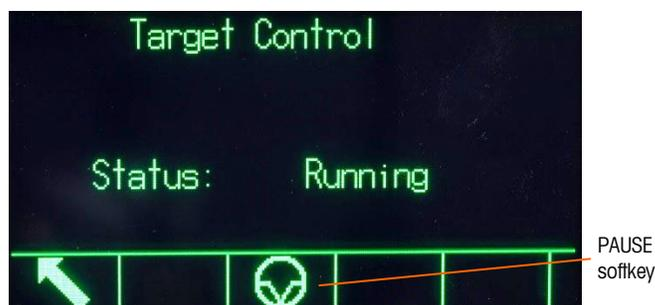
**Figure 2-20: Example of Running State in Target Control**
