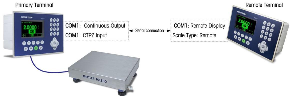
**Figure 2-18: Remote Display Function via Serial Communication**
