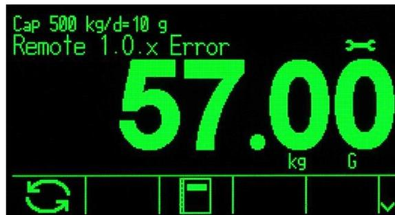
**Figure 2-38: Asynchronous Error System Line Message**
