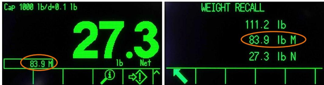
**Figure 2-15: Tare Displays with Net Sign Correction Enabled**
