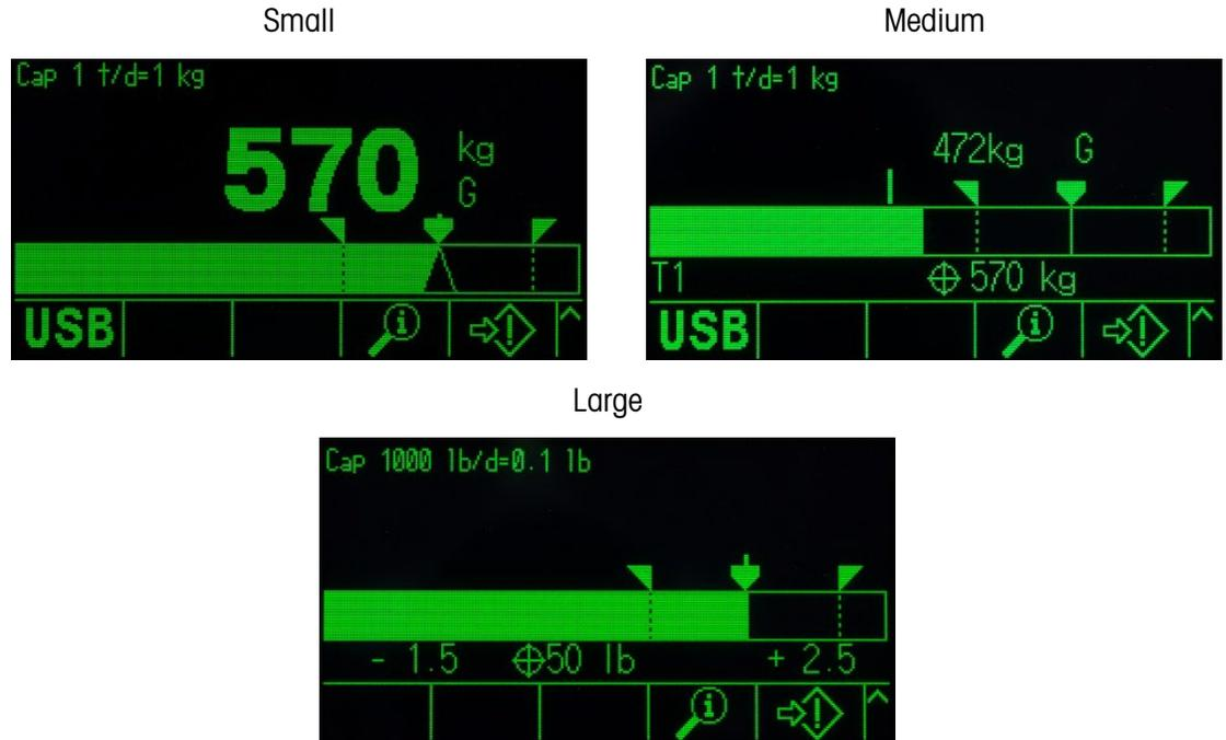
**Figure 4-18: SmartTrac Display Sizes in Material Transfer Mode**
