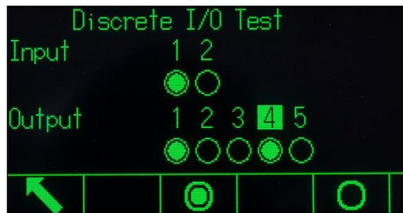
**Figure 5-16: Discrete I/O Test Screen**
