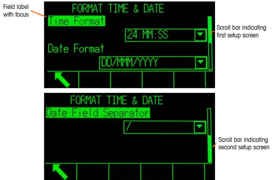
**Figure 3-3: Examples of Setup Screens (Format Time & Date)**
