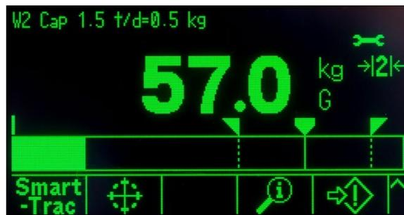
**Figure 1-11: Small Material Transfer SmartTrac Enabled**
