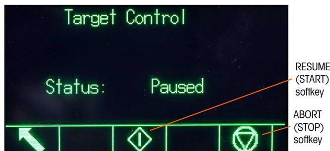
**Figure 2-21: Example of Paused State in Target Control**
