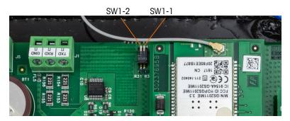
Figure 2-1: IND256x Metrology Switch Location
