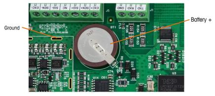
Figure 4-4: Battery Test
