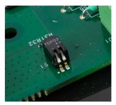
Figure 4-7: Metrology Switches SW1-1 and SW1-2, Both ON
