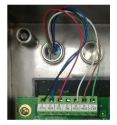
Figure 4-3: Analog Load Cell Connection Terminal
