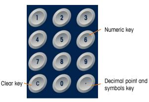
Figure 2-5: Numeric keyboard layout
