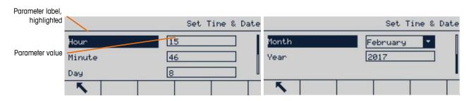
Figure 3-4: Setup Screen Example (Time and Date Setting)
