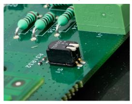
Figure 4-9: Metrology Switches SW1-1 and SW1-2, Both OFF
