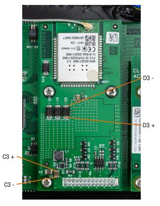
Figure 4-5: Testing positions for Wi-Fi board
