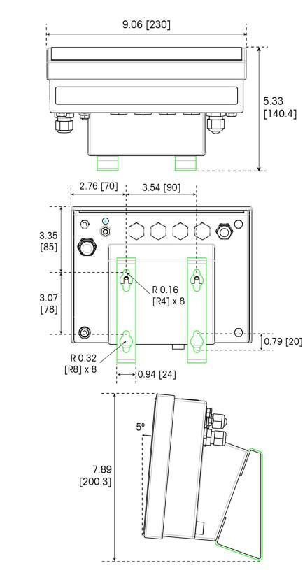
Figure 1-4: IND256x Dimensions, with Fixed Wall-Mount Bracket
