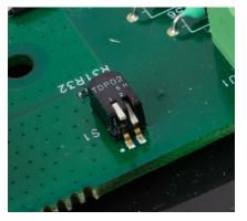
Figure 4-6: Metrology Switches SW1 OFF, SW2 ON
