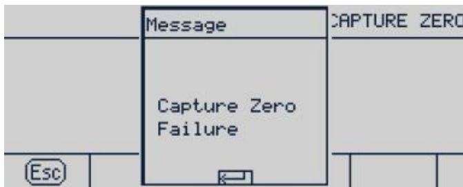
Figure 3-13: Zero Calibration (Failed)
