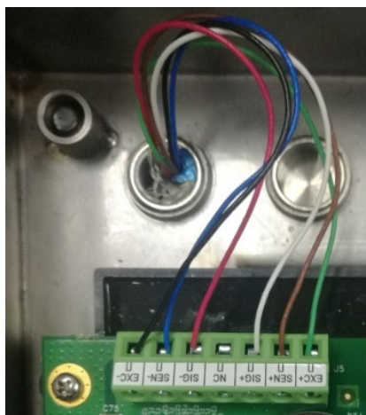
Figure 4-3: Analog Load Cell Connection Terminal
