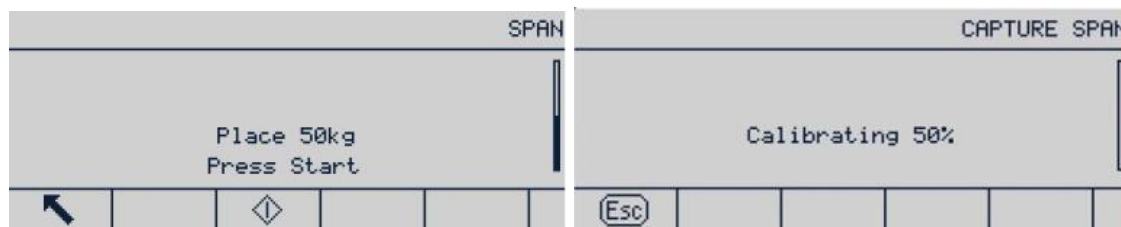
Figure 3-15: Span Calibration in Progress
