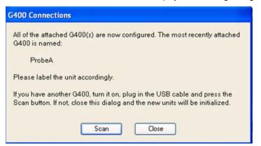
**2.** Plug in the other G400 USB cable and click the **Scan** button. After a few seconds, the second G400 will be configured and the dialog box updated with information identifying the new probe.
