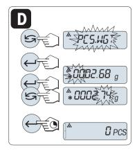
**Important:** If without any key press within 60 seconds, the balance return to the previous active application. Press **C** to cancel and returns to the previous active application.
