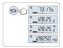
Press key at any time to switch the display between percent display, weighing unit UNIT 1, RECALL value (if activated) and weighing unit UNIT 2 (if different from UNIT 1).
