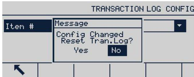
**Figure 3-52: Transaction Log Reset Screen**
