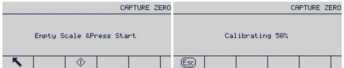
**Figure 3-11: Zero Calibration**
