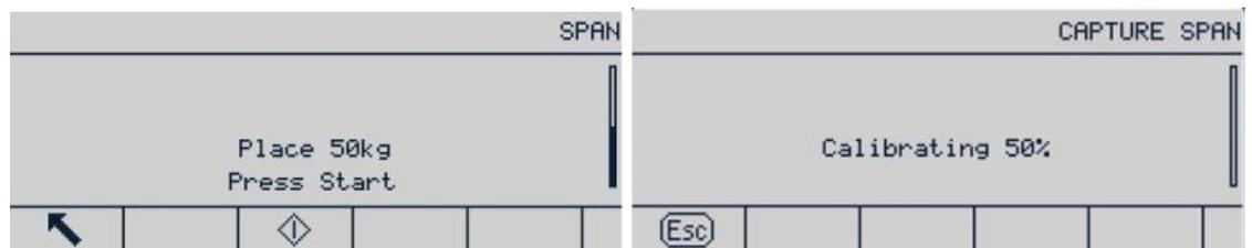
**Figure 3-15: Span Calibration in Progress**
