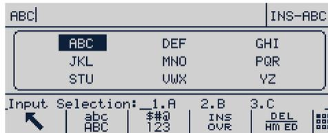
**Figure 2-7: Alphanumeric Input Screen**
