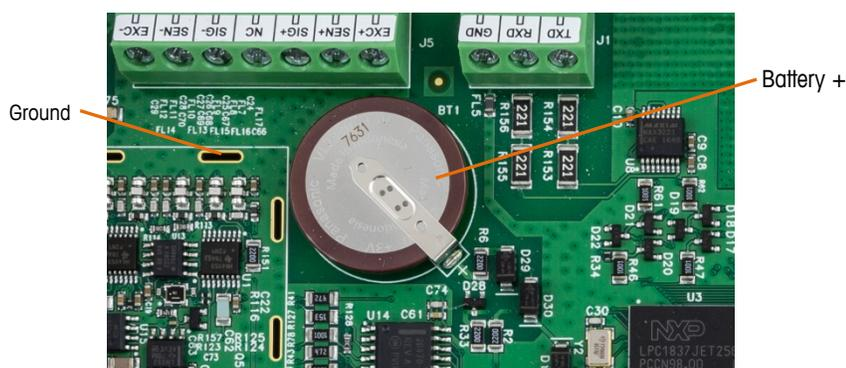
**Figure 4-4: Battery Test**
