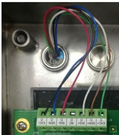
**Figure 4-3: Analog Load Cell Connection Terminal**
