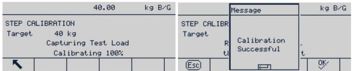
**Figure 3-24: Step Calibration Sequence**
