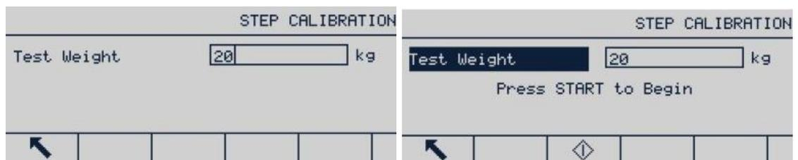
**Figure 3-22: Entering Test Weight Value**
