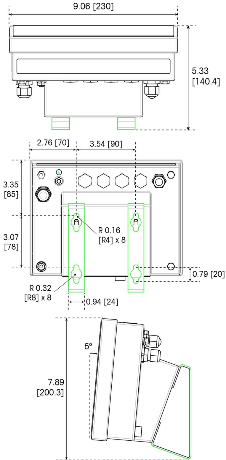
Figure 1-4: IND256x Dimensions, with Fixed Wall-Mount Bracket
