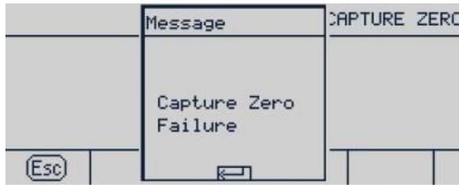
**Figure 3-13: Zero Calibration (Failed)**
