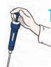
**1** First, after preparing the beaker and taring the balance, adjust the pipette to 100 percent of its nominal volume and load the manufacturer's recommended tip.
