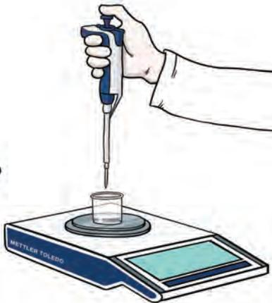
**6** Repeat the process three more times using the same tip, recording the mass each time.
