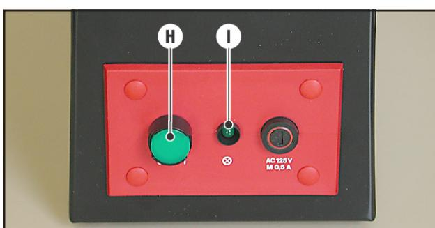
On/Off switch (H); control lamp (I) lit when the ionizer is active.
