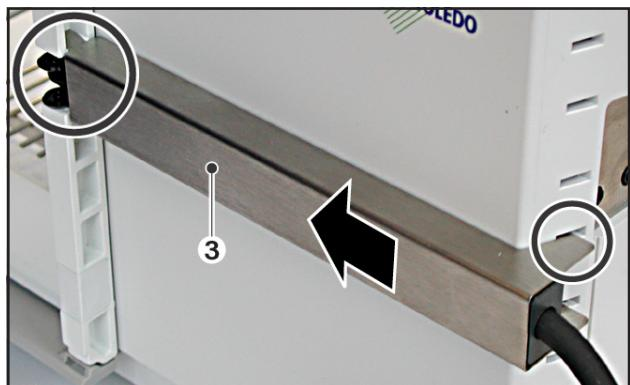
③ Push the point ionizer in from the back. If necessary, slightly bend the strips so that the ionizer is held firmly.
