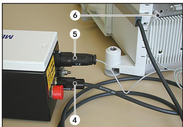
④ Screw the ionizer cable tightly onto the AC adapter.
