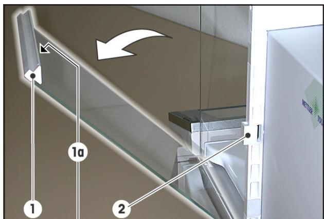
① Swap the side door for the door (marked with "Conducting Glass" 1a) supplied with the antistatic kit.
