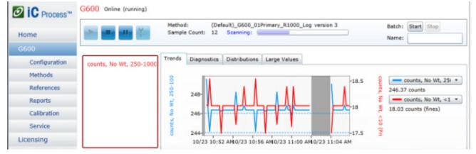
Figure D-1 Error display from alarm limits set in method
