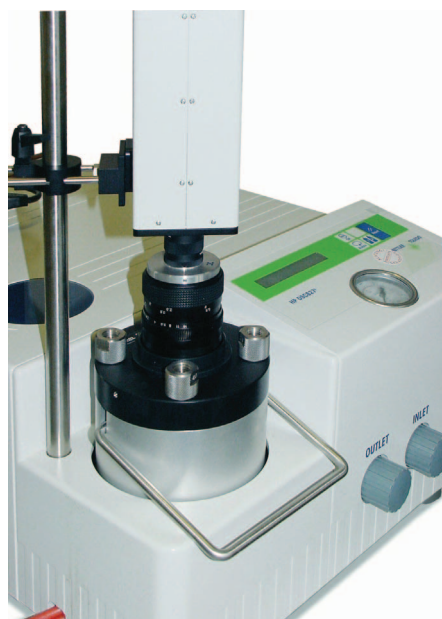
Fig. 2. HP DSC827 e with the chemiluminescence accessory.
