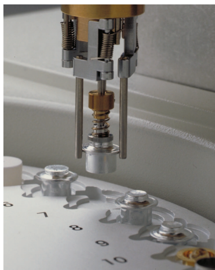
Fig. 1. The sample robot is equipped with a needle that pierces the special aluminum lid immediately before the measurement.
