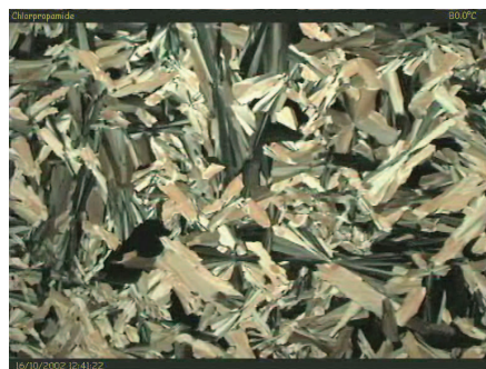
Fig. 7. Chlorpropamide crystals cooled from 135 °C at 10 K/min and then held isothermally at 80 °C.
