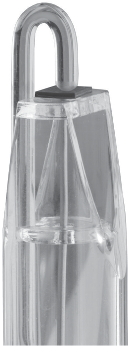
Fig. 3. Quartz glass sample support with the K-type thermocouple for sample temperature measurement.
