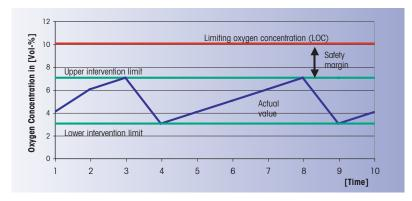
mal while safe operation is ensured. Depending on individual process conditions and solvent concentration, the oxygen level is maintained between 1 and 9 vol %.
