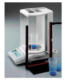
How charges originate. How does an electrostatic charge come into being? When an object is rubbed, an electrostatic charge is left behind. This can happen when a volumetric flask is held with tweezers, or a glass beaker dried with a cloth. Because many weighing containers are made from insulating material, this charge can only dissipate slowly, or not at all. Samples can even charge themselves, especially when being transferred or dispensed. This particularly applies to powders and granulates.
