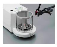
For every sample: the point ionizer. When powdery samples are electrostatically charged a draft is often enough to blow the substance into the air. With toxic substances this is highly problematical. In this case the point ionizer is the ideal solution. It discharges even the smallest objects. Its probe with a diameter of approx. 25 millimeters can also be inserted into the inside of containers. Thanks to its flexible cable, you can fasten the point ionizer in any position simply and easily.
