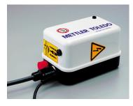
For both ionizers: the power pack. The high-voltage power pack with protection type IP54 and protection class I has two high-tension sockets. You can use them to connect both the U ionizer and the point ionizer. A function control built into the power pack indicates faults on an LED display. The patented coaxial plug connection guarantees safe assembly and disassembly in seconds without tools.
