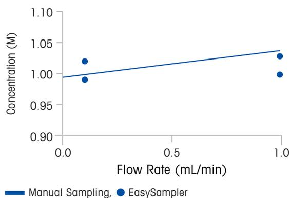
**Figure 3:** Comparison of 20 µL sampling from 1.0 M solution using EasySampler and manual pipette
