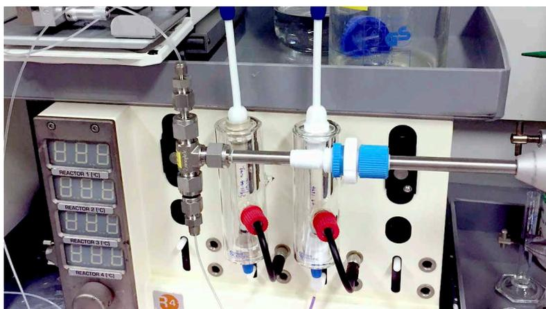
Figure 2: EasySampler connected to a flow reactor
