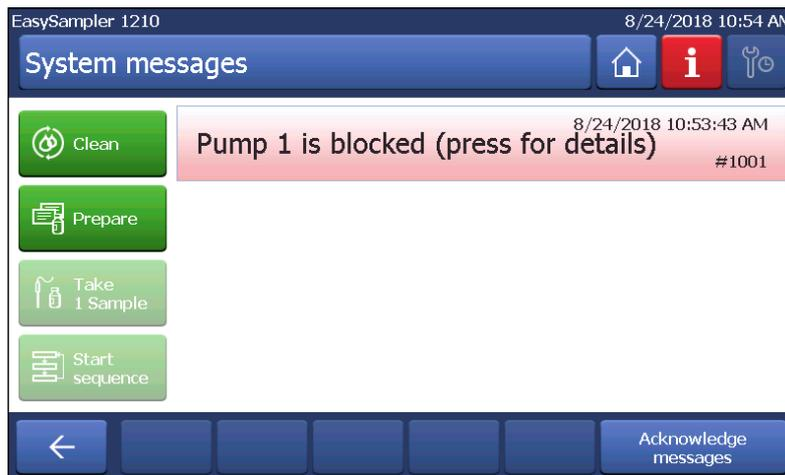
If the pressure in the fluidic system of EasySampler exceeds a certain level, the EasySampler pump is stopped to prevent any damage to the sleeve or the rest of the system.
