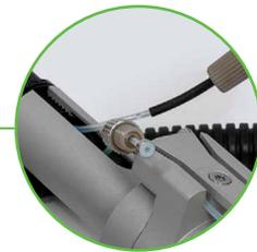
Disconnect the solvent tubes in the conduit from the probe and connect the syringe with the adapter to one of the tubes. Place the other end into a vessel and flush solvent through it. Repeat these steps for the second tube.
