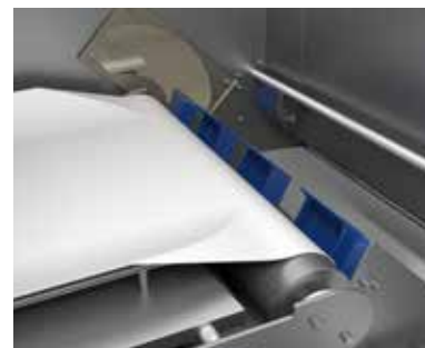
An example of a six lane scoop reject with three scoops up and three scoops down.
