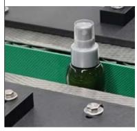
Side grip belts with special drives ensure safe and smooth transfer of the product to the inspection system and then on to the adjoining conveyor belt.
