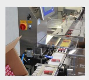
The packaging system's Overall Equipment Effectiveness (OEE) may be impacted if products are difficult to convey e.g. tubes. At the same time, inspection systems should be designed for the throughputs required and still have capacity left for future growth.
