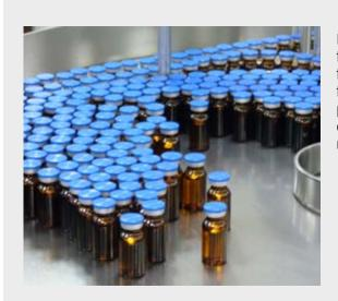
In addition to ensuring prescribed quantity tolerances are observed, modern weighing technology also detects over and underfilling tendencies at an early stage for liquid pharmaceutical products. Here, advanced software algorithms continuously analyse the weighing results and if necessary, readjust the filling station.
