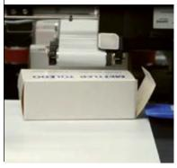
If the system detects boxes with open flaps or sloping angles, the checkweigher software receives a signal from the light barrier and tracks the position of the boxes. As these products can cause bottlenecks and line stoppages, they are separated before reaching the checkweigher's unloading conveyor belt, which increases the reliability of the line.
