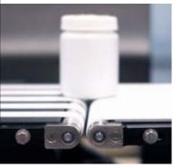
Unlike conventional conveyor belts connected in series, D15 conveyors use small 15mm pulleys to prevent lightweight products and items with small contact surfaces from getting stuck, turning or wobbling at the transition point and potentially disrupting the process.
