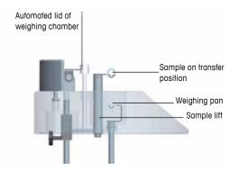
Step 1: loading of sample on the sample lift.
