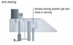
Step 2: moving the sample into the weighing chamber
