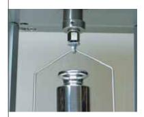
An optional adapter allows to weigh suspended loads below the weigh module. Overload protection is still assured in all directions.
