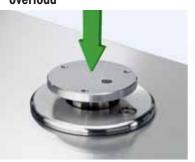
The weighing cell benefits from mechanical protection against vertical static overload of between 25 and 50 times the weighing capacity. This protects the weigh module in the event of malfunction of handling devices or mistakes during installation.
