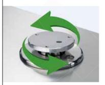
The pan is blocked against unwanted rotation in order to keep holding devices in position. However, the blockade opens in the event of collisions with handling devices, so that the pan can be turned through its own axis without risk of damage.
