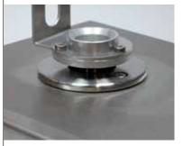
The weighing pan has three holes to fasten customized adapters to hold vials or tubes. An adapter may weigh 1/3 of the full load without restricting weighing capacity. The pan can be lifted off the weigh module without having to use tools.
