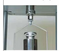
An optional adapter allows to weigh suspendeed loads below the weigh module. Overload protection is still assured in all directions.
