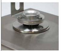
The weighing pan has three holes to fasten customized adapters to hold vials or tubes. An adapter may weigh 1/3 of the full load without restricting weighing capacity. The pan can be lifted off the weigh module without having to use tools.
