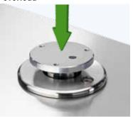
The weighing cell benefits from mechanical protection against vertical static overload of between 25 and 50 times the weighing capacity. This protects the weigh module in the event of malfunction of handling devices or mistakes during installation.
