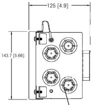
2 Hole plugs supplied to close any unused cable entry fittings.
