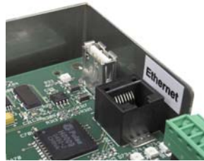
Figure 2-3: IND780 Ethernet Port
