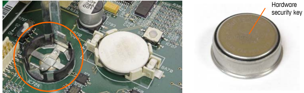
Figure 1-2: IND780 Hardware Key Socket on Mother Board
