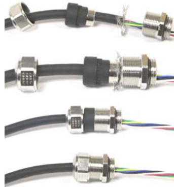
Figure A-24: Installing Metal Cable Gland with Shield Wire
