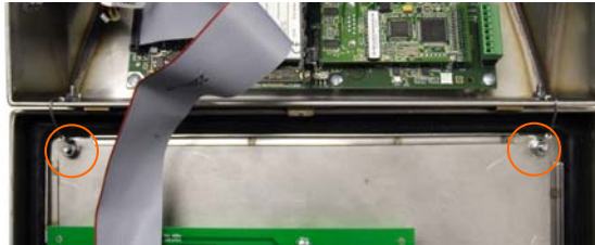
Figure A-7: Ground Strap Attachment Locations
