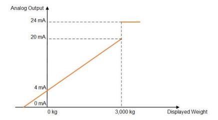
The analog output signal can be calibrated via the Analog Output Adjustment submenu. ACT100/ACT100xx can increase or decrease the analog signal via two levels of adjustment (Coarse and Fine adjustment).
