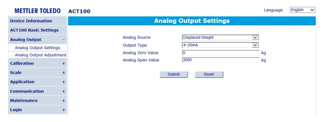
For example, if the Output Type is set as  $4\sim20$  mA, Analog Zero Value as 0 kg and Analog Span Value as 3,000 kg, ACT100/ACT100xx will output 4 mA when the scale is empty (0 kg) and 20 mA when 3,000 kg load is on the scale. In this case, when live weight exceeds 3,000 kg, the analog output signal will jump from 20 mA to 24 mA as a warning to the DCS/PLC.
