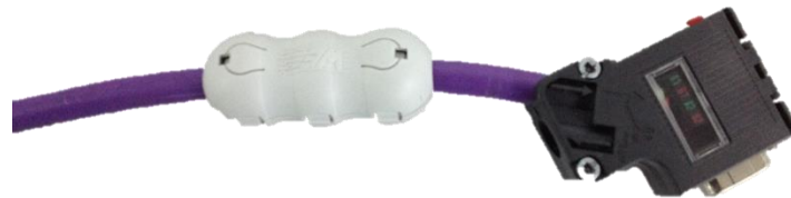
Figure 3-13 Ferrite Installed on PROFIBUS DP Cable
