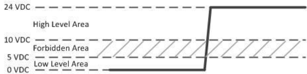
Figure 3-6 A Rising-edge Trigger Signal on Input
