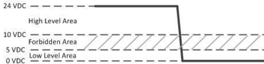
Figure 3-7 A Falling-edge Trigger Signal on Input
