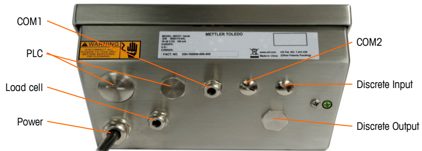
Figure 2-25: Harsh Enclosure Gland Assignments
