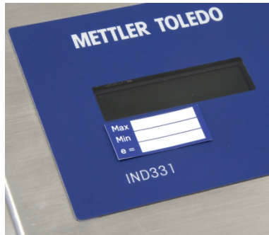
Figure 2-80: Capacity Label Location, Harsh Unit
