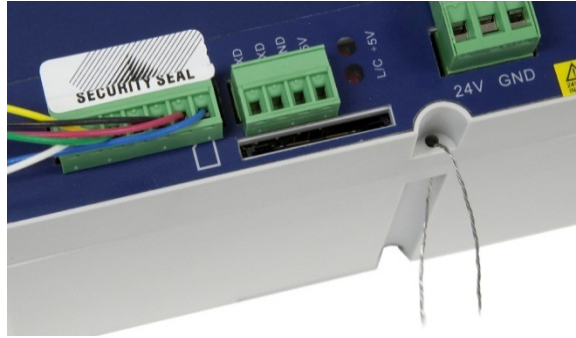
Figure 2-82: DIN and Panel-Mount Sealing – Wire and Paper Seals
