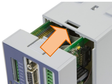
Figure 2-74: Snapping the Cover into Place
