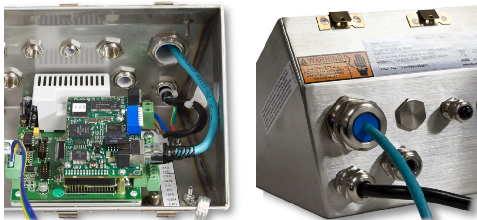
Figure 2-66: Ethernet Cable Routing – harsh Enclosure
