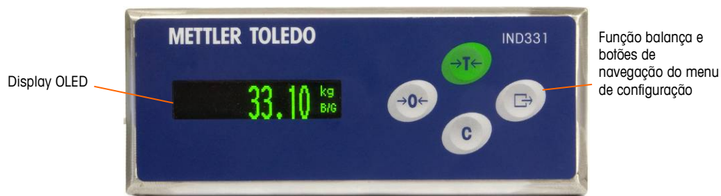
Figura 1-9: Layout de painel frontal IND331
