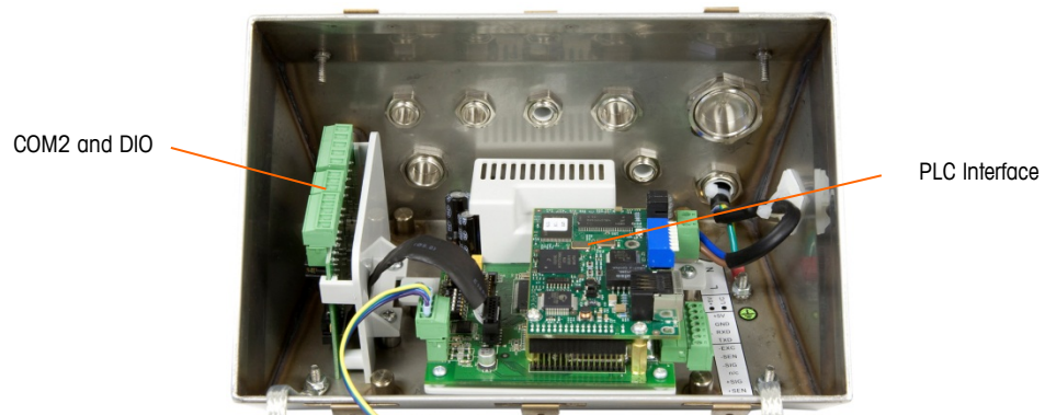
Figure 2-43: Option Locations in the Harsh Enclosure
