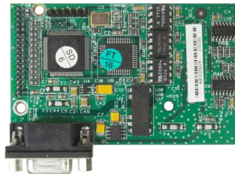
Figure 2-67: PROFIBUS Option Board, Panel Mount Enclosure
