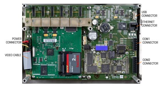
Figure 4-9: Main PCB Connections and Mounting Screws
