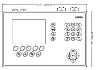
Figure 1-3: Harsh Environment Enclosure Dimensions, Front
