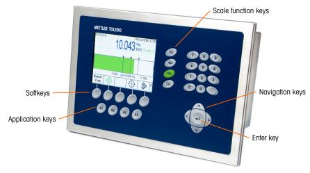
Figure 1-5 shows the IND780's display and keyboard layout.
