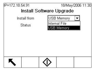
Figure 4-1: Firmware Upgrade From USB Memory
