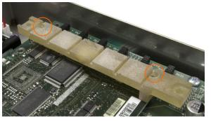
Figure 4-51: Lower Card Guide Screw Locations
