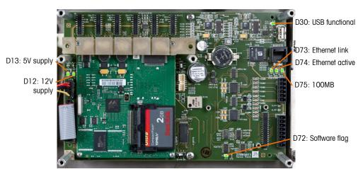
Figure 4-4: Main PCB LEDs
