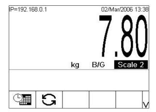
Figure 2-15 shows the Home screen with primary units (kilograms) displayed.
