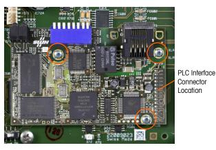
Figure 4-60: PLC Interface Module Installed on Main PCB
