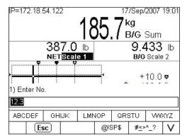
Figure 2-24: Two Scales plus Sum with SmartTrac and ID Sequence Display
