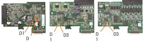
Figure 4-6: &ED Locations: IDNet (left), Serial (center) and DIO (right) Cards
