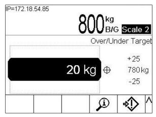
Figure 2-30: Example of Over/Under Display
