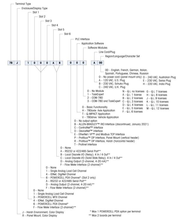
Figure 1-1: IND780 Model Identification Numbers
