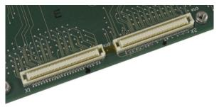
Figure 4-53: Close-Up View of ETX Connectors on Main PCB
