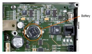
Figure 4-11: Main PCB, Battery Location Indicated
