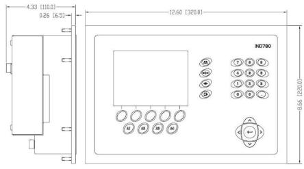
Figure 1-2: IND780 Panel Mount Enclosure Dimensions
