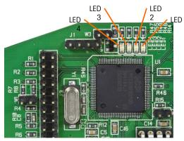
Figure 4-8: Analog Output Board LEDs
