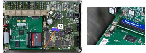
Figure 2-1: Metrology Switch, Location (left), shown in its OFF position (right)
