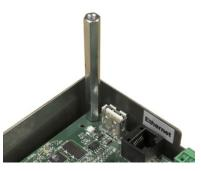
Figure 4-49: Stand-Off on Main PCB
