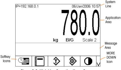
Figure 2-9: Weighing Operation Home Screen
