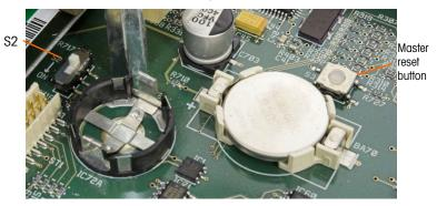
Figure 4-46: Main PCB, Master Reset Button and S2 Locations Indicated
