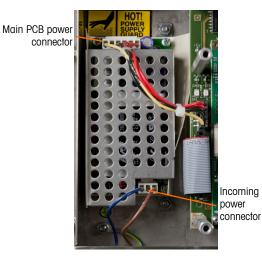
Figure 4-58: Power Supply, Connected
