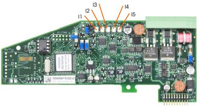
Figure 4-7: Board LEDs
