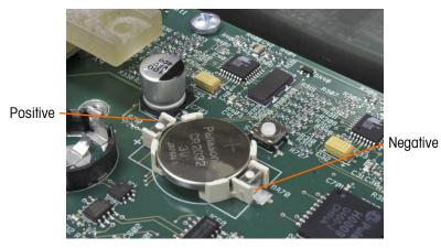
Figure 4-12: Battery Installed
