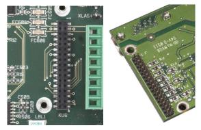
Figure 4-61: PLC Interface Module Socket on Main PCB (left) and Connector Pins on the Underside of a Module (right)
