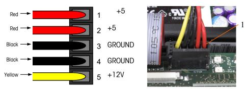
Figure 4-10: Pins on the Power Supply Harness
