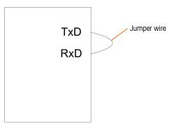
Figure 4-24: Jumper Wire Placed Between the Transmit and Receive Terminals
