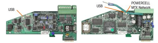
Figure 4-5: Analog Load Cell (left) and POWERCELL MTX (right) LEDs
