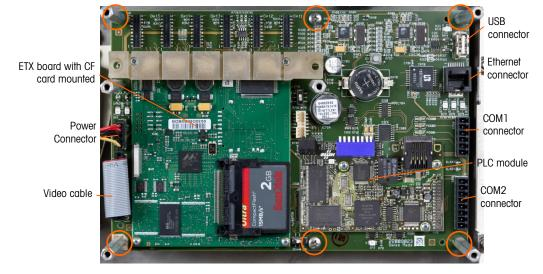
Figure 4-48: Main PCB Connections and Mounting Screws
