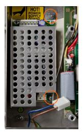
Figure 4-59: Power Supply, Disconnected
