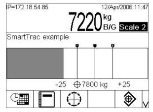
Figure 2-28: Bar Graph, Large SmartTrac Display
