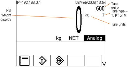
Figure 2-14 Screen Displaying Captured Tare
