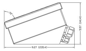
Figure 1-4: Harsh Environment Enclosure Dimensions, Side
