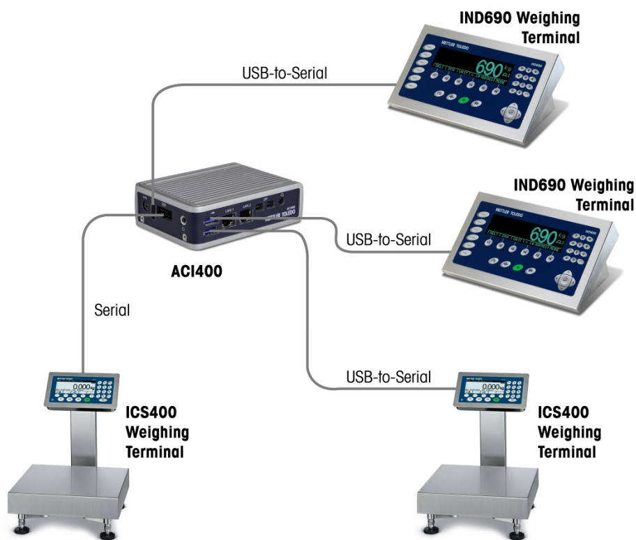
Figure 1-6: ACI400 with IND590s and ICS400s
