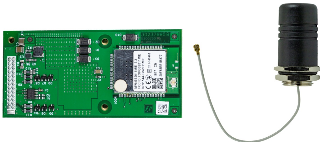
Figure 2-14: IND256x WiFi Option Board and Antenna
