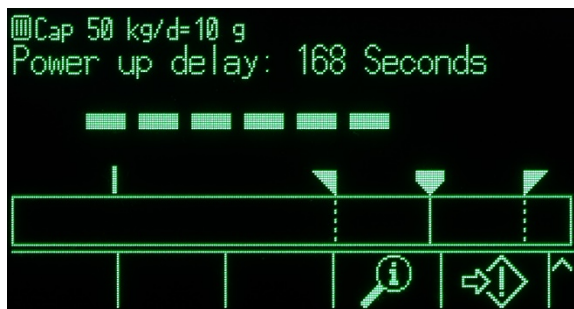
Figure 3-6: Power Up Delay Shown in System Line
