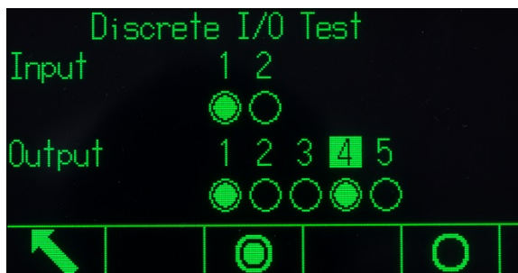
Figure 5-16: Discrete I/O Test Screen
