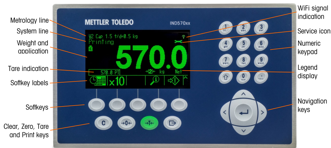
Figure 1-10: IND570 Front Panel Layout
