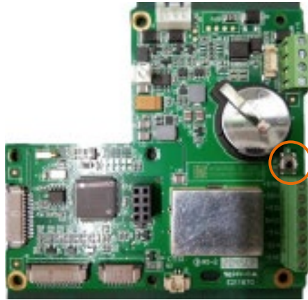
Figure 3-2: Setup Switch Location on Terminal Main Board
