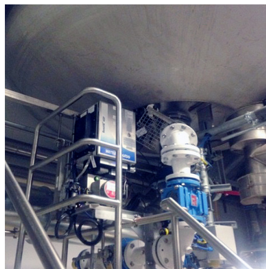
Figure 1. Picture of the process ReactIR 45P at the bottom of the tosylfuranoside reduction vessel (15,000 L). Mid-IR operation is continuous 24/7. Photo courtesy of Roche Clarecastle, Ireland.
