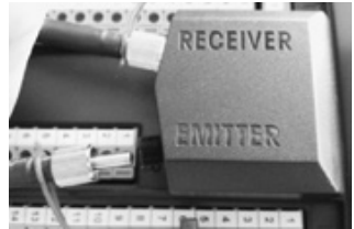
Fig. 4: SMA-connection to M800 transmitter "Receiver/Emitter".
