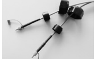
Fig. 2: Gaskets mounted on fiber optic cable.
