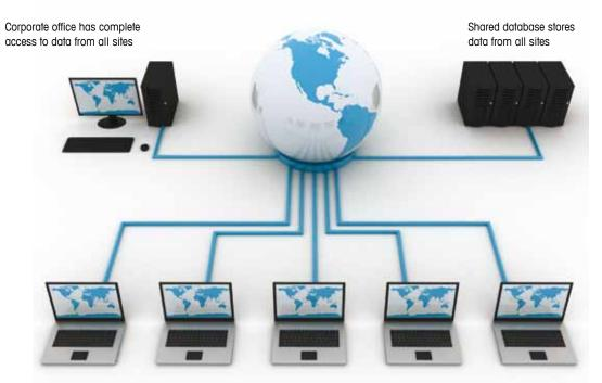
Install DataBridge™ ES software at a corporate office and DataBridge™ MS software at multiple sites with multiple workstations
