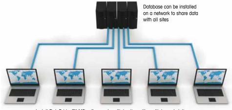
Install DataBridge<sup>TM</sup> MS software at multiple sites with multiple workstations (each workstation controls as many as six vehicle scales)
