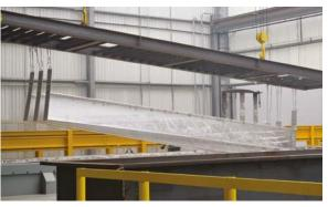
Hot-dip galvanizing coats the steel surface with a protective layer of zinc. By dipping the steel in a bath of molten zinc, the process covers the steel components completely, inside and out. Galvanized steel provides maintenance-free corrosion protection for the life of your scale.
