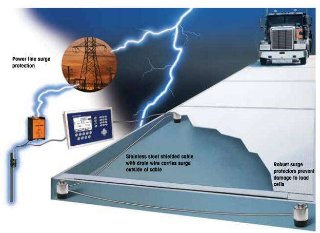
Single-point ground provides path of least resistance away from electronics
