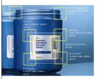
Vision inspection systems ensure that products consistently meet manufacturers' exacting quality standards and specifications.
