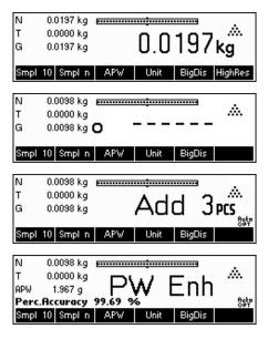
10 samples were placed on the scale and **«Smpl 10»** was pressed.
