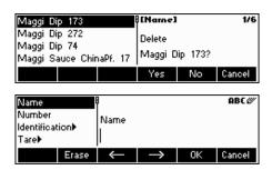
Press «**Delete**» to remove the current article from the database. You will be asked to confirm deletion of an article.
