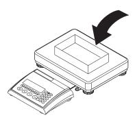
Place the **empty** weighing container or packaging on the platter and then press the  $\leftarrow$ T  $\leftarrow$  » key briefly, or press the  $\leftarrow$ PT » softkey if a **known tare** weight has already been established.
