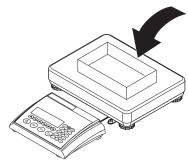
Place the **empty** weighing container or packaging on the platter.
