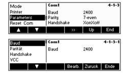
The current Baud Rate, Parity and Handshake settings are displayed on the screen.
