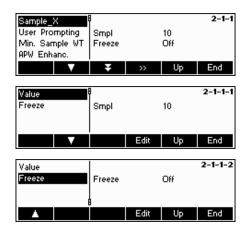
Press « >>> to change the settings into the desired number of pieces or to freeze the actual setting of the Smpl X value.
