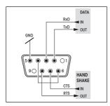
Every balance can be equipped with an optional RS232C interface for connection to a peripheral device (e.g. printer, auxiliary display or PC with a 9-pin male connector, see Section 6.4). The balance must then configured to suit the peripheral device in a menu dialog (Sections 4.3.8 - 4.3.13).
