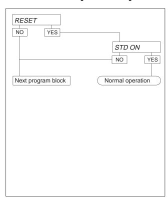
The program block RESET allows you to reset any parameters changed in the master mode to the default or standard factory settings at a keystroke.
