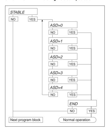
In this block you can match the automatic stability detector to meet your individual requirements. The settings change the time taken by the weighing platform to recognize stability.
