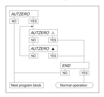
When the weighing platform is unloaded, the autozero function automatically compensates the weight of small amounts of dust or other contaminants. This block offers the possibility to switch the autozero correction on or off to suit your requirements.
