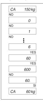
The maximum capacity shown in the display does not correspond to the desired value. Reply with NO.
