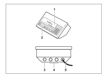
The weighing terminal comprises the following components:
