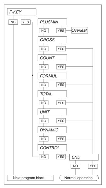
In this program block you can assign one of the following functions to the  $\neg$ Fe key:
