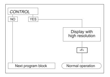
In the program block CONTROL, you can increase the resolution of the display for test purposes.
