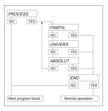
In this program block you can match the display of the weighing terminal to the weighing sample.
