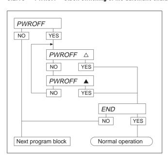
If the automatic shutdown is activated, the scale switches itself off automatically when no weight has been loaded for 10 minutes.
