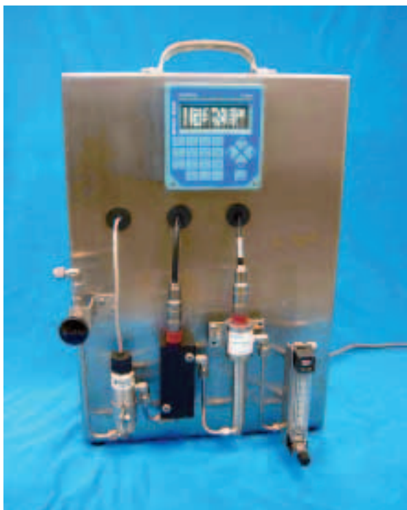
Figure 2: THORNTON 770MAX with sensors for conductivity, dissolved oxygen and pH.
