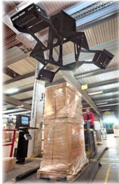
CSN840 Pallet™ is a complete data capture solution with dimensioner, scale and bar code reader.
