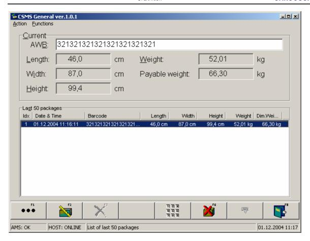
III-b. If any measurement is wrong, a dialog box shows the reason for the measurement not beiing Ok.
