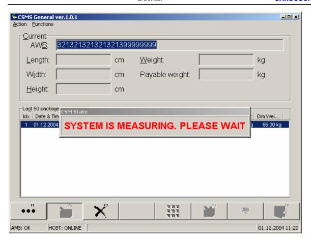
III-a. If all measurements are Ok, all fields are greyed and will stay on the screen until the next AWB is read. However, the operator will see that the measurements have popped up in the Last 50 packages field.
