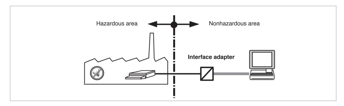
The **interface adapter** allows the attachment of nonintrinsically safe peripheral instruments in the nonhazardous area to intrinsically safe scales of the SMx series in the hazardous area.
