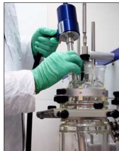
Lasentec® FBRM® and PVM® technologies are directly installed in a LabMax® automated lab reactor for in-process measurement of the crystal product.
