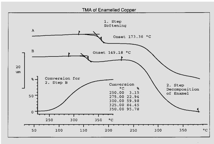
The diagram shows the experimental curves of two copper wires (A and B) insulated with different enamels. In principle, the same behavior is apparent, namely softening of the insulation recognizable from the 1<sup>st</sup> step at around 150°C and the subsequent thermal decomposition as the 2<sup>nd</sup> step.
