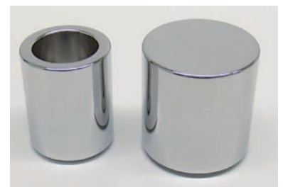
Density determination with Buoyancy Artefacts
