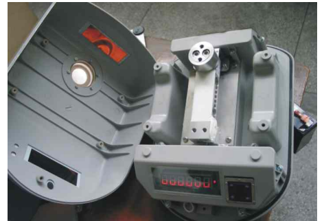
Dual enclosures with water-proof sealing
