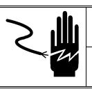
DISCONNECT ALL POWER TO THIS UNIT BEFORE INSTALLING, SERVICING, CLEANING, OR REMOVING THE FUSE. FAILURE TO DO SO COULD RESULT IN BODILY HARM AND/OR PROPERTY DAMAGE.
